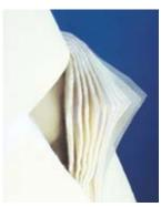
use bags, where performance levels previously required cartridges. These Graded Density Bags are made of multiple layers of microfibers and standard fibers variably calendered, providing filtration to 1 micron. Heavy-duty handles for ease in removal are a standard feature. The fully shaped bottoms enhance the pressure capacities of the bag. THE 500 SERIES HAS 9 LAYERS OF MICROFIBER MATERIAL, EACH WITH 4.4 SQ. FT. OF SURFACE AREA.
